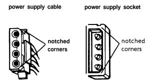
You must connect a power supply cable to each drive you install in your system. If you'll be reinstalling a hard disk drive in the vertical mounting position, connect the power supply cable to this drive first. If not, connect the power supply cable to the drive you just installed in the lower horizontal drive bay.
